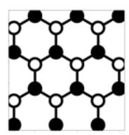
The layers are stacked such that on top of each boron atom there is a nitrogen atom in the next layer and vice versa, as shown in the plot below. The distance between neighboring B and N atoms within each layer is a, the distance between the layers is h.
